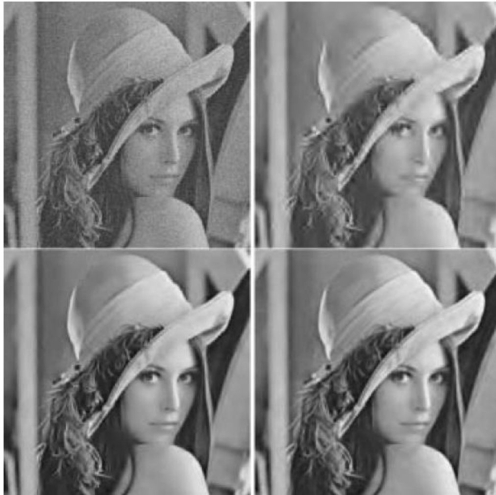
Fig. 5. (Top left) Noisy image and (top right) filtered images using the decimated wavelet transform, (bottom left) the undecimated wavelet transform and the (bottom right) curvelet transform.
